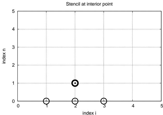
Figure 2: Modified stencil for the first time step.
