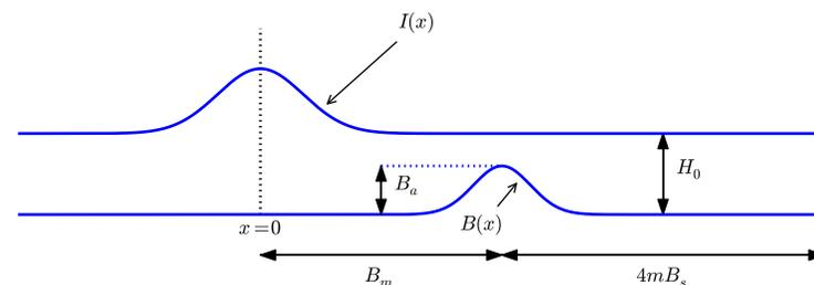
Figure 11: Sketch of an earthquake-generated tsunami passing over a subsea hill.
