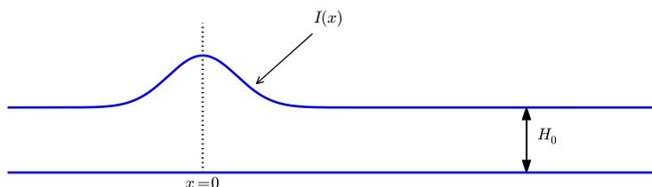
Figure 9: Sketch of initial water surface due to a subsea earthquake.
