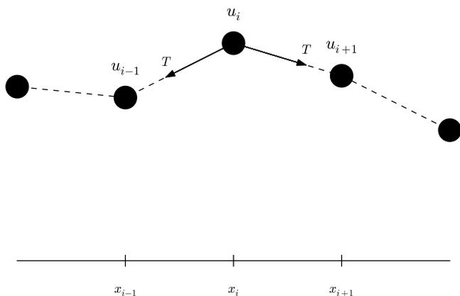
Figure 8: Discrete string model with point masses connected by elastic strings.
