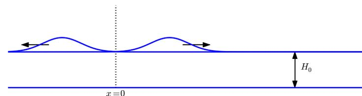
Figure 10: An initial surface elevation is split into two waves.
