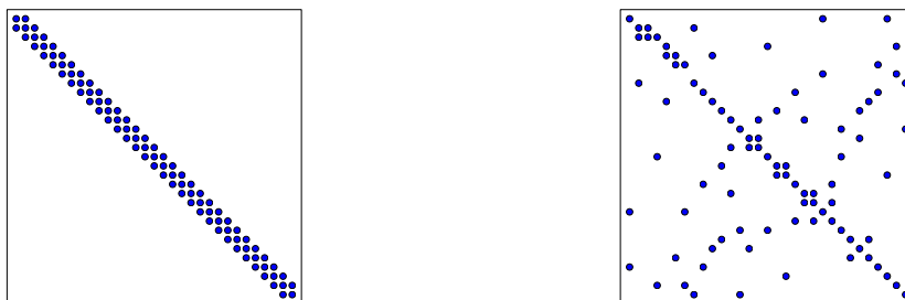
Figure 32: Matrix sparsity pattern for left-to-right numbering (left) and random numbering (right) of nodes in P1 elements.
