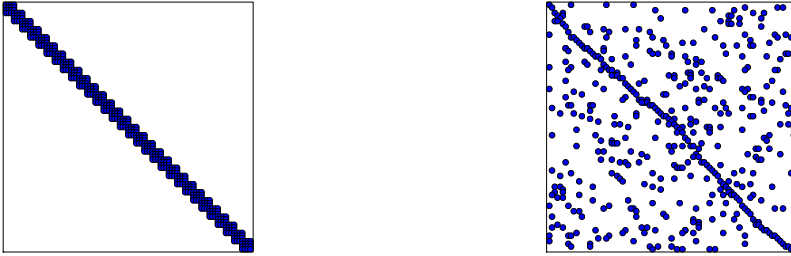
Fig. 3.19 Matrix sparsity pattern for left-to-right numbering (left) and random numbering (right) of nodes in P3 elements.
