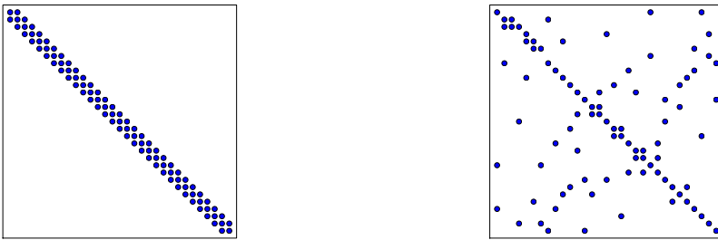
Fig. 3.18 Matrix sparsity pattern for left-to-right numbering (left) and random numbering (right) of nodes in P1 elements.
