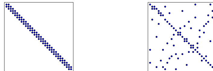
Figure 30: Matrix sparsity pattern for left-to-right numbering (left) and random numbering (right) of nodes in P1 elements.
