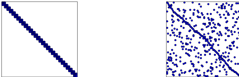
Figure 31: Matrix sparsity pattern for left-to-right numbering (left) and random numbering (right) of nodes in P3 elements.
