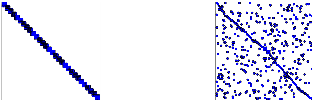
Figure 31: Matrix sparsity pattern for left-to-right numbering (left) and random numbering (right) of nodes in P3 elements.
