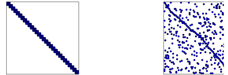
Figure 31: Matrix sparsity pattern for left-to-right numbering (left) and numbering (right) of nodes in P3 elements.
